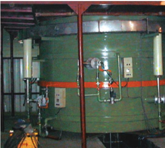
*Direct heating of a bell furnace for annealing.
